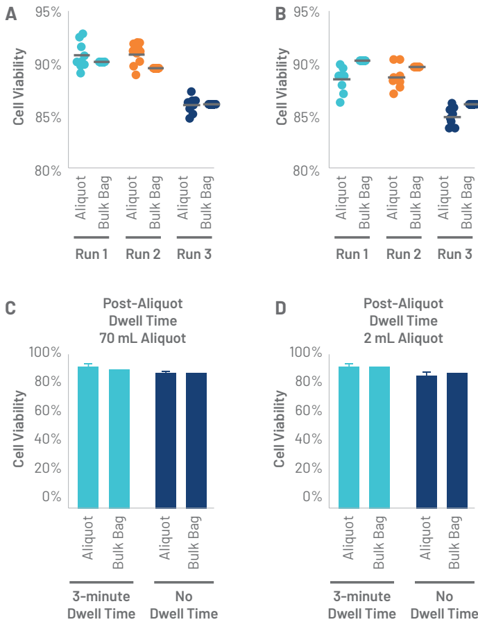
Figure 3: Cell viability of each aliquot measured by AOPI stain. The horizontal line indicates the average cell viability (A and B). Post-aliquot dwell time does not impact cell viability when comparing a procedure including a 3-minute post-aliquot pause (Dwell Time) versus a procedure with no pause configured (No Dwell Time). Error bars indicate mean with SD (C and D).
